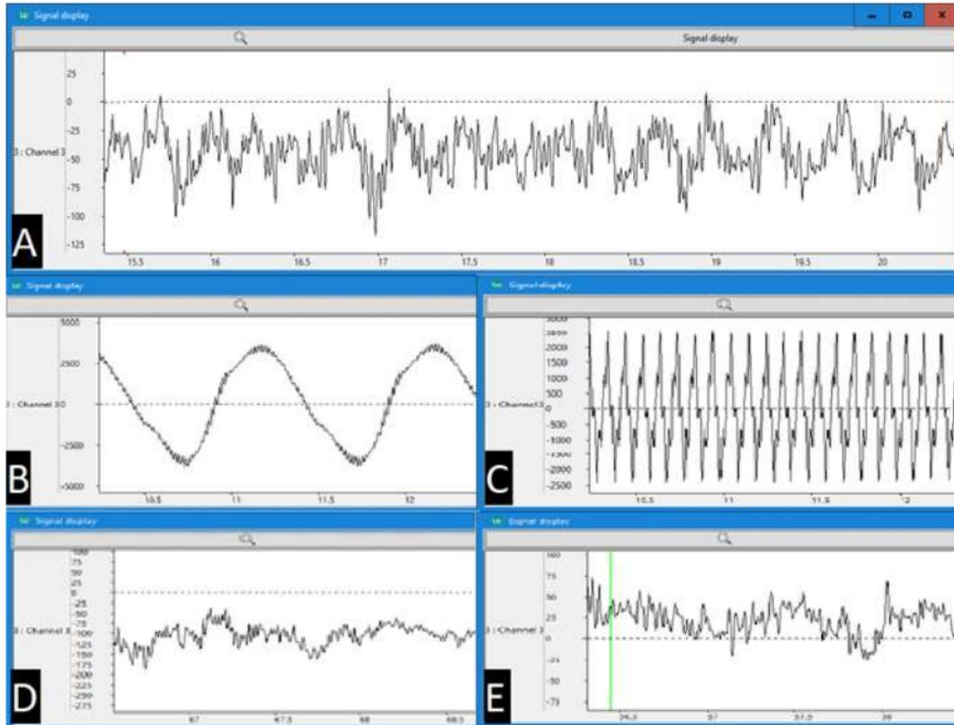
**Fig. 4:** EEG measured signal: A. without ECVT excitation, B. with 1 Hz excitation, C. with 10 Hz excitation, D. with 100 Hz excitation and E. with 200 Hz excitation
