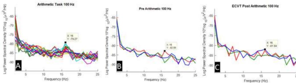
Fig. 6: PSD of ECVT signal during: A. arithmetic task, B. pre-arithmetic task and C. post-arithmetic task.
