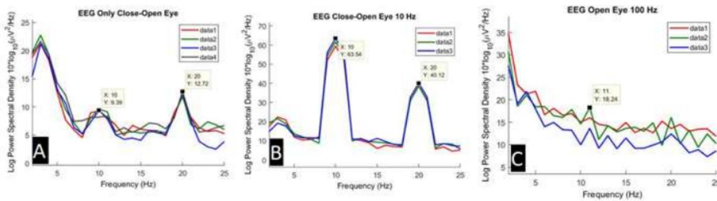
**Fig. 5:** PSD of EEG signal during relax condition: A. without ECVT excitation; and with B. 10 Hz and C. 100 Hz ECVT excitation.
