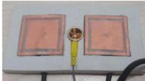
Fig. 1: An integrated Brain ECVT and EEG sensor.
