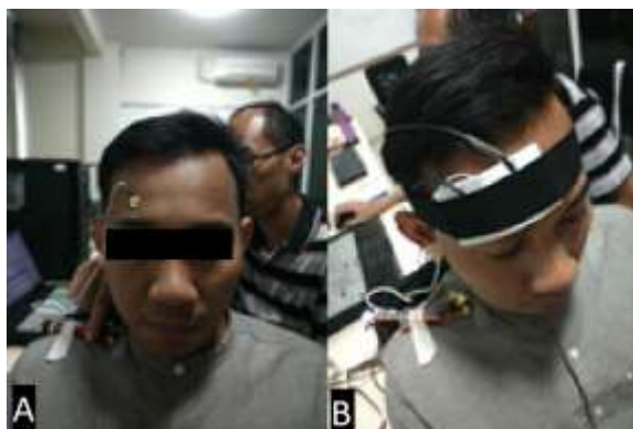
Fig. 2: The sensor placement on the subject's Fp2 location: A. EEG electrode and B. integrated ECVT-EEG sensor
