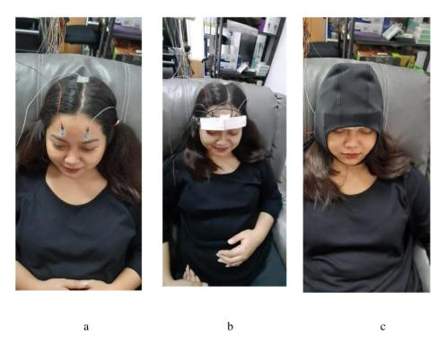
Figure 2. Integrated EEG-ECVT sensor placement on the subject's head.
