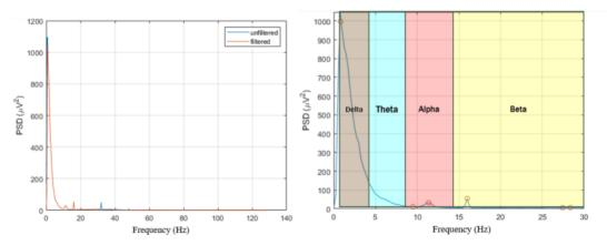
Figure 2. (a) Unfiltered and filtered power spectral density (b) Spectral features: 6 peaks locations showed in red bullet and brain frequency range (delta, theta, alpha, beta)
