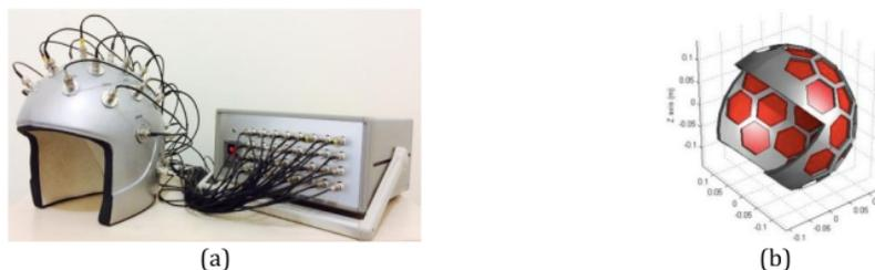
**Figure 1** (a) Helmet sensor of Brain ECVT and DAS; (b) Sensor configuration
