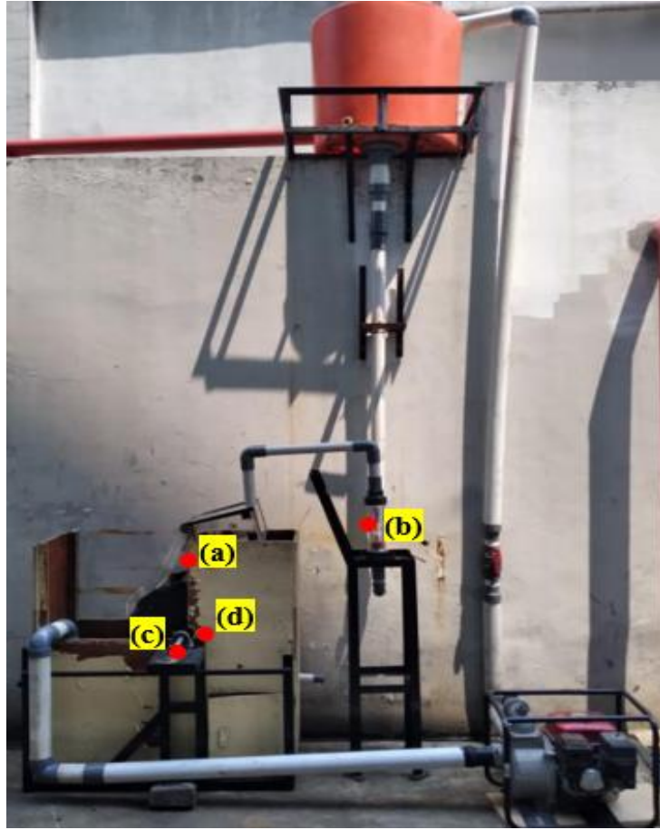
Fig. 5. The assembled overshot waterwheel installation and data collection location. (a) water flow velocity data, (b) water discharge data, (c) waterwheel torque data, and (d) waterwheel rotation data
