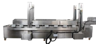
Gambar 46. Sistem kontinyu (Sumber: http://m.id.hibestcoatingmachine.com/frying-machine/small-medium-large-continuous-industrial.html )
