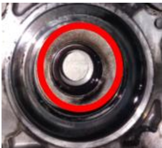
Figure 27. Damaged fuel pump parts.
