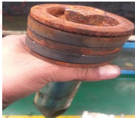
Figure 68. Pneumatic piston corrosion
