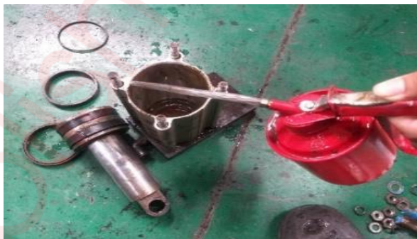
Figure 72. Wetted pneumatic parts with ISO VG 32 oil
