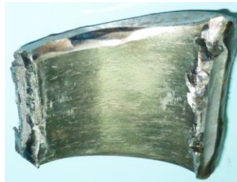
Figure 49. Small end (rod eye) fracture shape in position B
