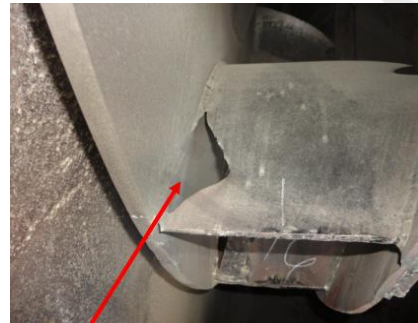
Figure 37b. IDF perforated blade
