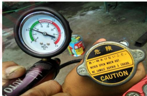
Figure 63. Radiator cap measurements
