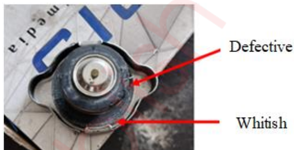
Figure 64. Damaged radiator cap seal and whitish color
