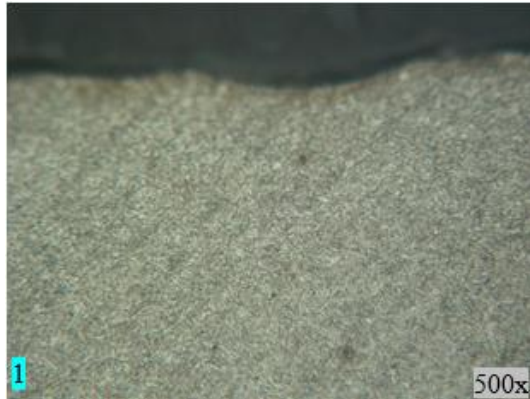
Figure 19. Microstructure of tampered martensite
