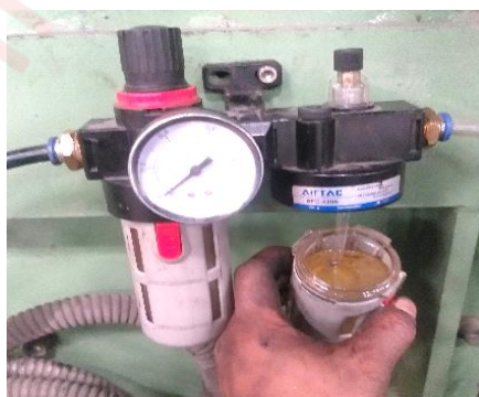
Figure 75. Filling the lubricator tube with ISO VG 68 lubricating oil
