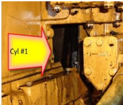
Figure 41. Broken cylinder engine block
