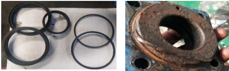
Figure 69. Damaged pneumatic seal
