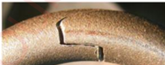
Figure 16. Broken shape of the injector spring
