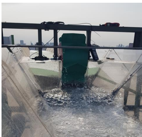
Fig. 1. Dethridge wheel experimental rig installation
