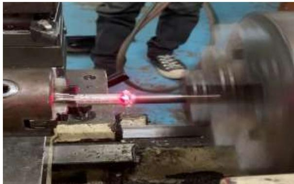
*Gambar 3. 5 Proses pengelasan friction welding*
