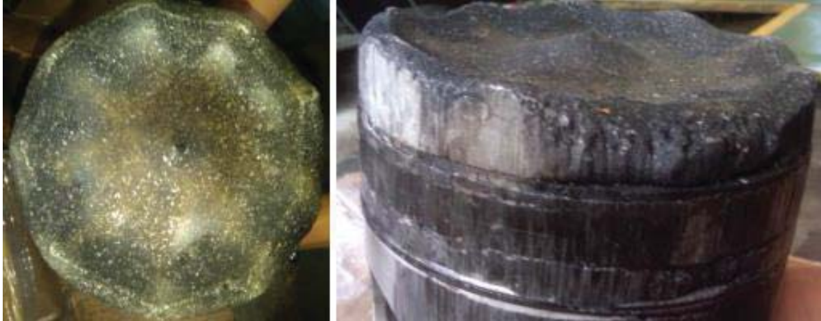
FIGURE 4. Top melting piston crown on cylinder # 12.
