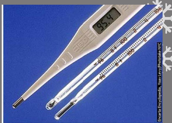
Gambar 123. Termometer Digital
