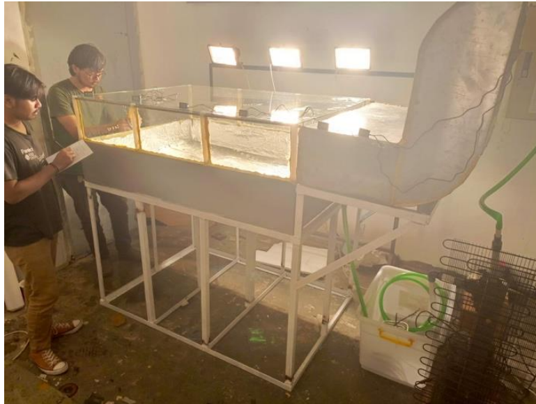
Fig. 1. Forced-flow desalination experimental rig
