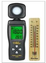
**Figure 1.** Lux meter and room thermometer
