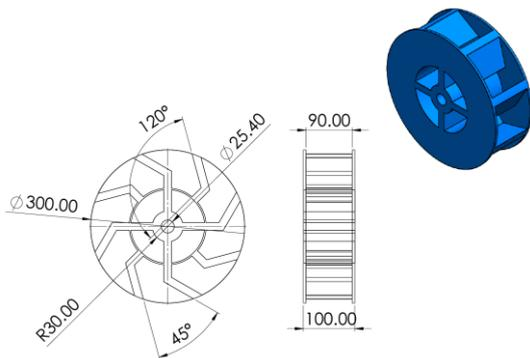
Figure 2. Waterwheel Dimensions
