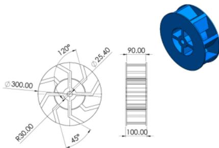
Figure 2. Waterwheel Dimensions
