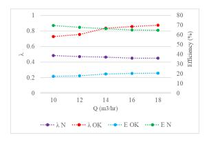
Figure 9. Efficiency Graph (%) and Tip Speed Ratio ( $\lambda$ )
