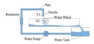
Figure 3. Nozzle Line Testing Installation
