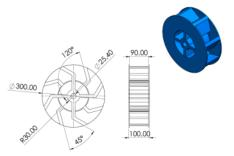
Figure 2. Waterwheel Dimensions
