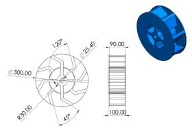
Figure 2. Waterwheel Dimensions
