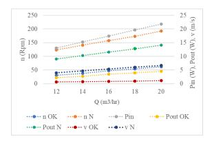
**Figure 7.** Graph of mill power (P <sub>out</sub>), mill power (P<sub>in</sub>), mill rotation speed (n), flow speed (v) and water discharge (Q)
