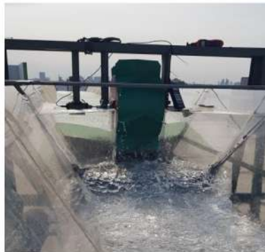
Fig. 1. Dethridge wheel experimental rig installation
