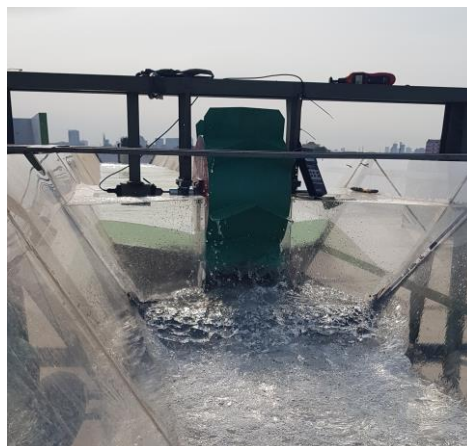
Fig. 1. Dethridge wheel experimental rig installation
