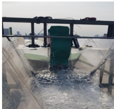
Fig. 1. Dethridge wheel experimental rig installation
