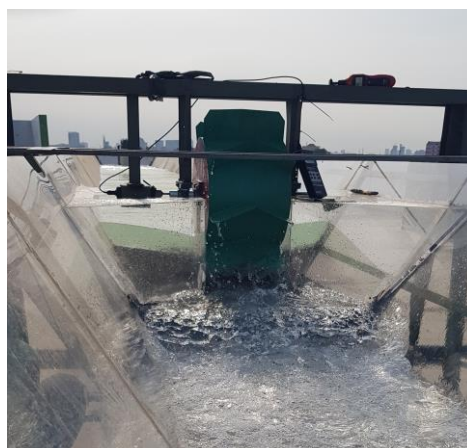
Fig. 1. Dethridge wheel experimental rig installation
