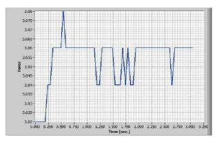
Fig. 5. Normal Force, Fn of 0.3 lbF is Exerted on the Splitter.
