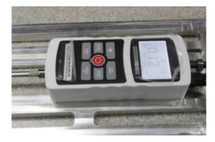
Fig. 3. Force Gauge used to Exert Pressure onto the Splitter.
