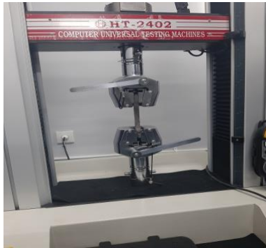
Figure 1. The HT-2402 tensile testing machine
