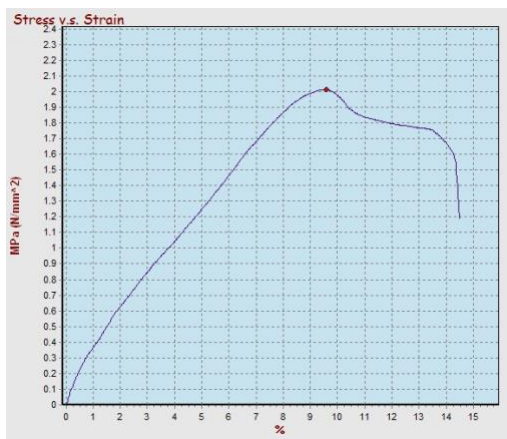
Figure 16. Tensile strength graph of sample KR50KS50
