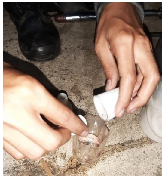
Figure 7. The process of mixing resin and catalyst
