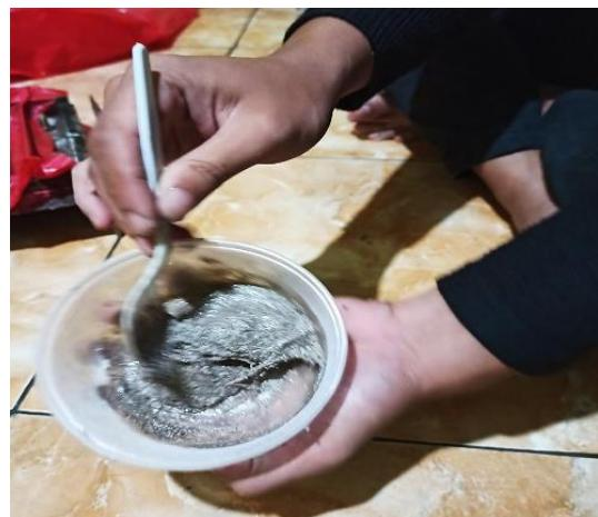
**Figure 6.** Mixing of brake pads and simping clamshells
