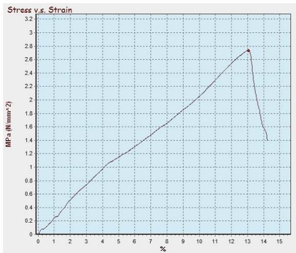
**Figure 14.** Tensile strength graph of sample KR40KS60
