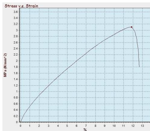
**Figure 17.** Tensile strength graph of sample KR100
