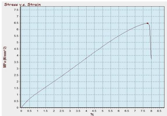
**Figure 12.** Tensile strength graph of sample KS100
