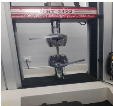
**Figure 1.** The HT-2402 tensile testing machine
