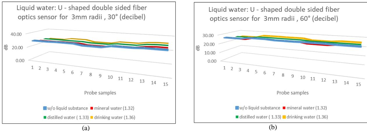
Figure 3. (a) and (b). Comparison results for pure water (dB) designed for 3 mm radii with polishing angle 30° and 60°.
