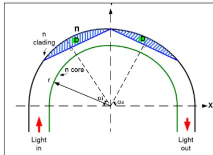
Figure 1. The schematic structure of the Double – Sided U – Shaped Plastic Optical Fiber.
