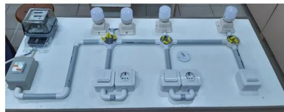
Gambar 1. Alat peraga instalasi listrik 1 phase
