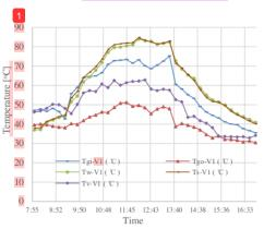
**Figure 9.** Temperature of basin water (Tw), vapour (Tv), inner side of cover glass (Tgi) and outer side of cover glass (Tgo) in control solar still on 1<sup>st</sup> September 2018
