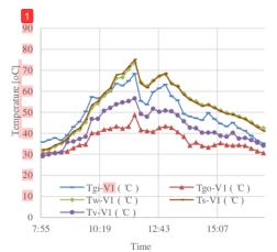
**Figure 7.** Temperature of basin water (Tw), vapour (Tv), inner side of cover glass (Tgi), and outer side of cover glass (Tgo) in control solar still on 29<sup>th</sup> August 2018
