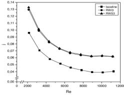
Fig 3. Graph of j values versus Re for in-line and staggered arrangements
