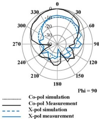
Fig. 9. Simulation and measurement result of SIFA radiation pattern at 4.8 GHz for  $\Phi = 90^\circ$
