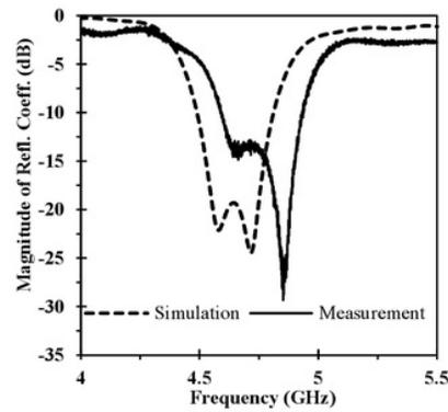
Fig. 7. Magnitude of reflection coefficient comparison between simulation and measurement.
