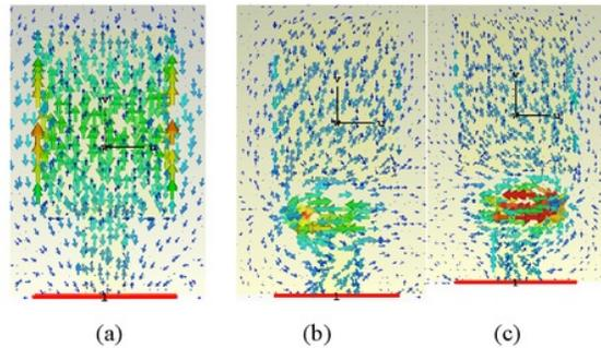
Fig. 4. The surface current of (a) conventional antenna (b) SIFA with via at the right arm (c) SIFA with via at the left arm
