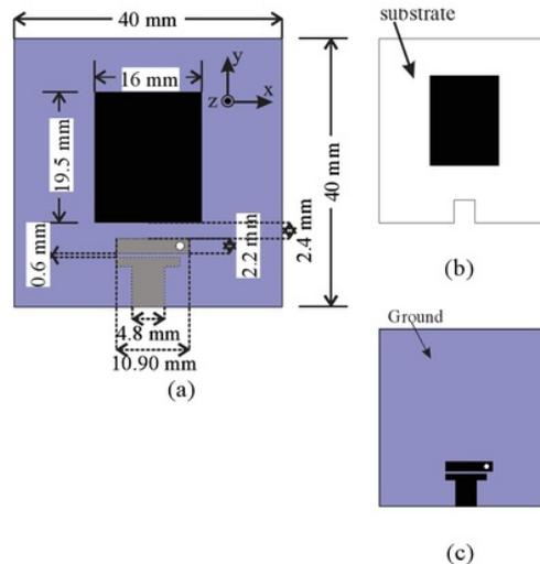
Fig. 1. Geometry of the stacked filtering antenna (a) Stacked Antenna (b) First layer (c) Second layer.
