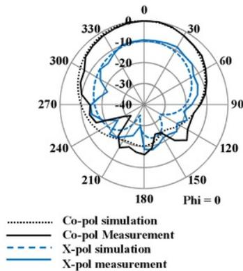
Fig. 10. Simulation and measurement result of SIFA radiation pattern at 4.8 GHz for  $\Phi = 0^\circ$
