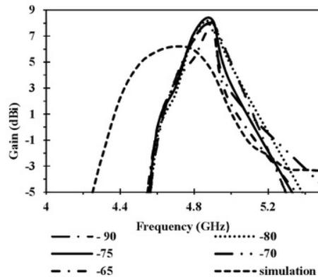
Fig. 8. Simulation and measurement result of SIFA Gain with various inclination of slant ( $\theta$ ) polarization
