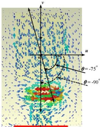
Fig. 5. SIFA with via on the left arm and its current surface inclination ( $\theta$ ) from the horizontal axis ( $+u$ ).
