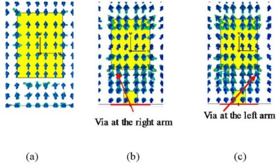
Fig. 3. The electrical field of (a) conventional proximity fed (b) via on the right hand (c) via on the left hand
