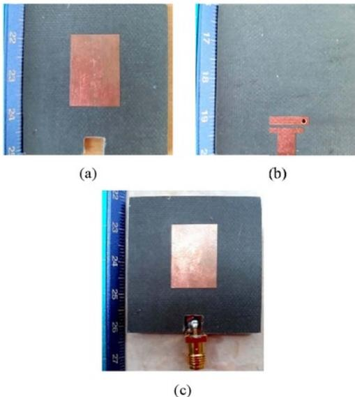
Fig. 6. The picture of prototype stacked interdigital filtering antenna (SIFA) (a) Rectangular radiator at the first layer (b) Interdigital resonator with via at the left arm at the second layer (c) Stacked Filtering Antenna.
