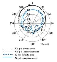
Fig. 10. Simulation and measurement result of SIFA radiation pattern at 4.8 GHz for Phi =  $0^{\circ}$
