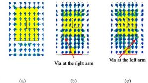
Fig. 3. The electrical field of (a) conventional proximity fed (b) via on the right hand (c) via on the left hand
