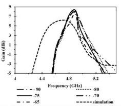
Fig. 8. Simulation and measurement result of SIFA Gain with various inclination of slant ( $\partial$  polarization
