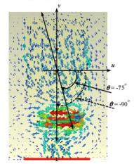
Fig. 5. SIFA with via on the left arm and its current surface inclination ( $\theta$ ) from the horizontal axis (+u).
