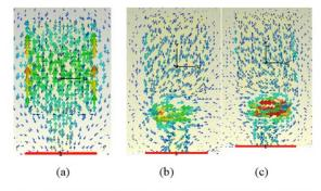
Fig. 4. The surface current of (a) conventional antenna (b) SIFA with via at the right arm (c) SIFA with via at the left arm
