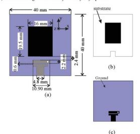
Fig. 1. Geometry of the stacked filtering antenna (a) Stacked Antenna (b) First layer (c) Second layer.
