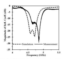
Fig. 7. Magnitude of reflection coefficient comparison between simulation and measurement.
