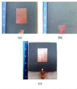
Fig. 6. The picture of prototype stacked interdigital filtering antenna (SIFA) (a) Rectangular radiator at the first layer (b) Interdigital resonator with via at the left arm at the second layer (c) Stacked Filtering Antenna.
