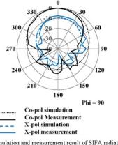
Fig. 9. Simulation and measurement result of SIFA radiation pattern at 4.8 GHz for Phi =90  $^{\rm o}$
