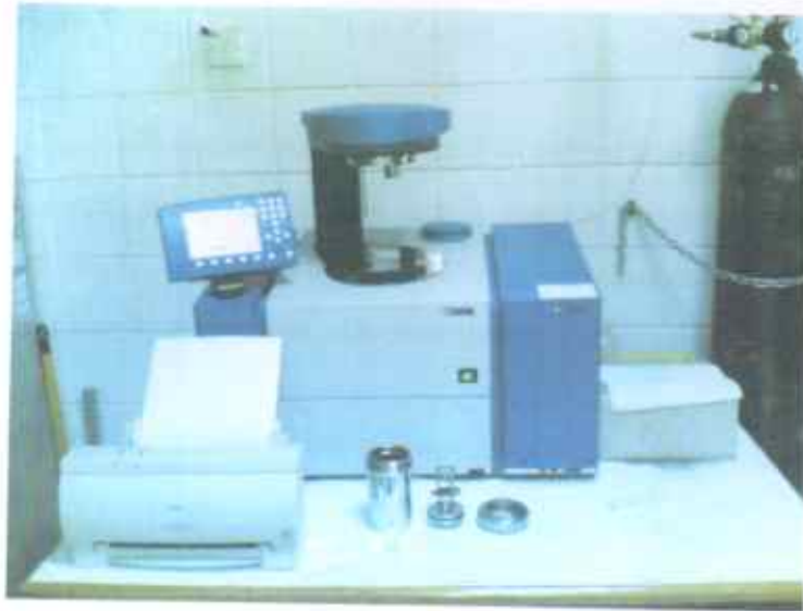
Rajah 3.9 gambar kalorimeter bom model kawalan C5000
