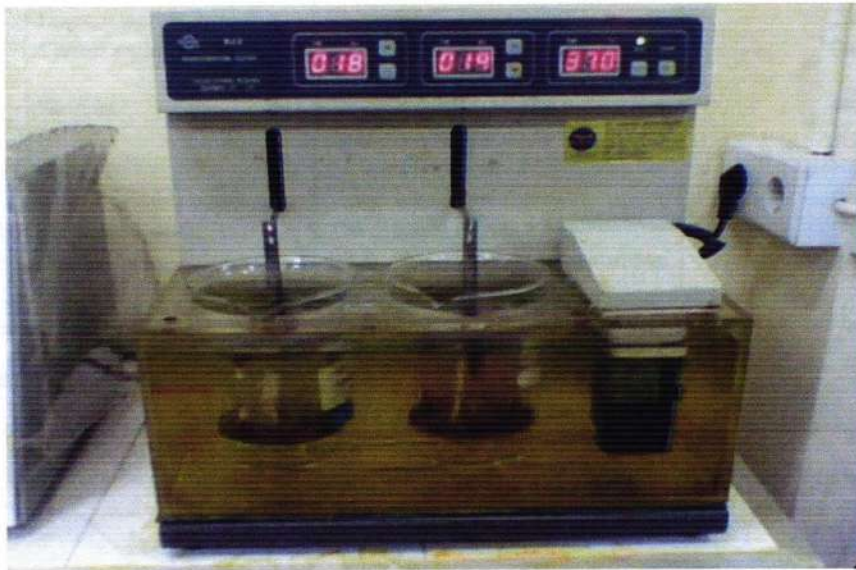
Gambar 29. Alat uji wash off ( desintegration tester )
