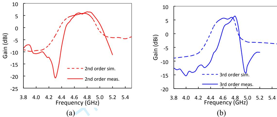
Fig. 7 (a) The Ant. I's gain comparison of simulation and measurement results, (b) The Ant. II's gain comparison of simulation and measurement results.
