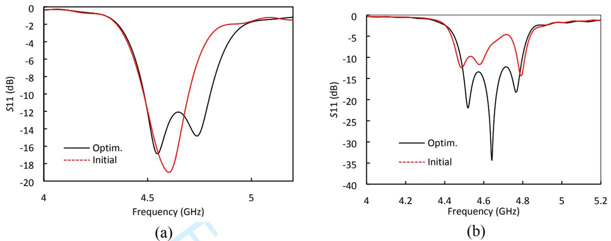
Fig. 5. (a) The initial and optimized design of second-order and (b) third-order interdigital filtering antenna.
