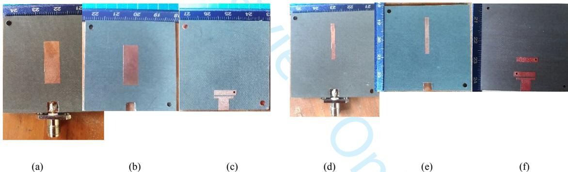
Fig. 8 Fabrication (a) assembled (b) radiator on the first layer (c) filtering circuit of Ant. I, (d) assembled (b) radiator on the first layer (c) filtering circuit of Ant. II
