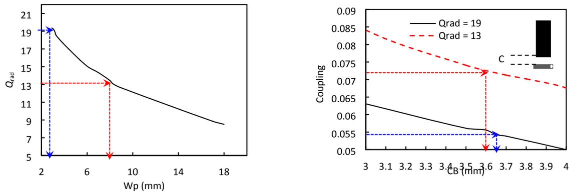
Fig. 4. (a) The extraction of  $Q_{\text{rad}}$  under different  $W_p$  and (b) coupling under different  $Q_{\text{rad}}$  and  $C_B$
