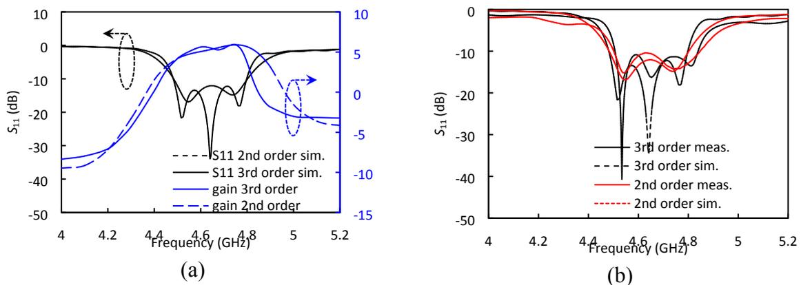
Fig. 6. (a) The optimized  $S_{11}$  and gain simulation comparison of the second-order and third-order and (b) the  $S_{11}$  measurement and simulation results comparison of the 2<sup>nd</sup> order and 3<sup>rd</sup> order filtering antennas
