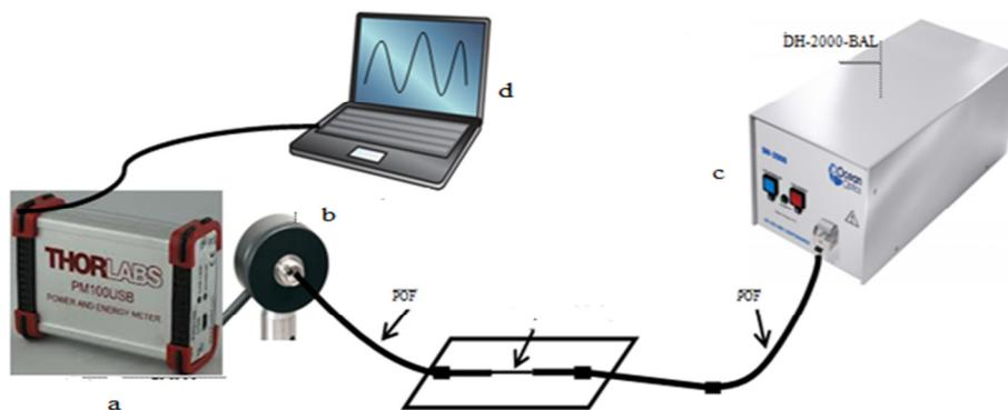
**Figure 1.** Experimental setup measurement of POF loss propagation of etching process:
