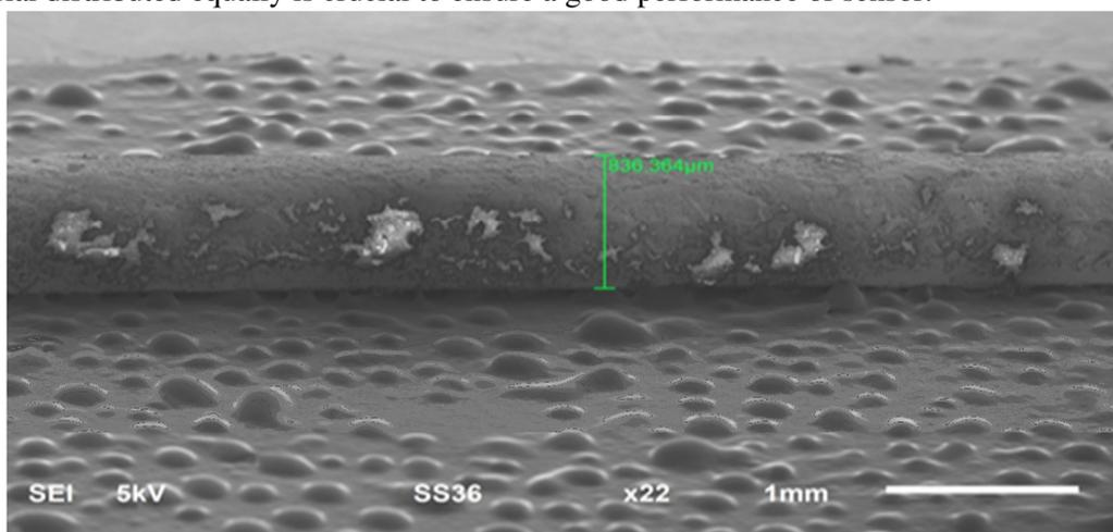
**Figure 5.** SEM image of POF coated with ZnO
