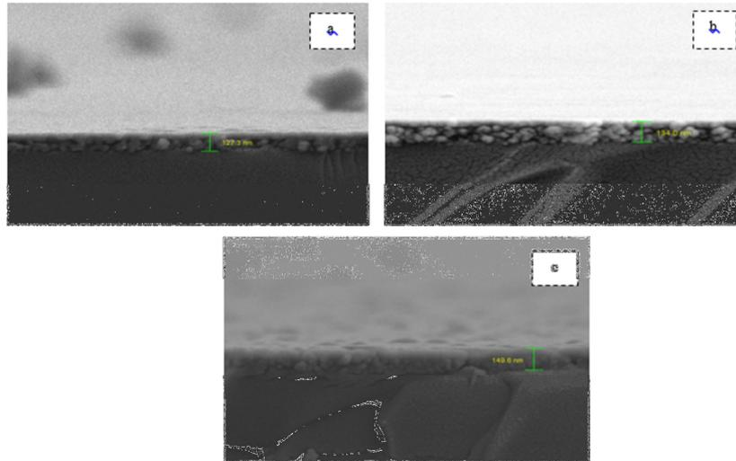
**Figure 6.** Scanning electron microscopy of the ZnO (a) 118nm (b) 134 nm (c) 149.06 nm
