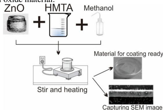
**Figure 2.** The synthesized process of ZnO as coating layer on the fibers using sol-gel method
