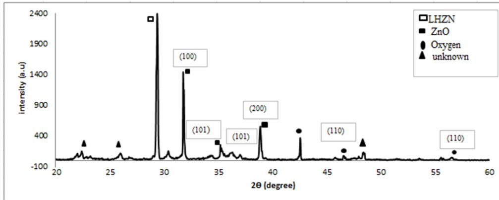
**Figure 4.** Typical XRD pattern of ZnO nanoparticles synthesized using solgel method (JCPDS 36-1451)
