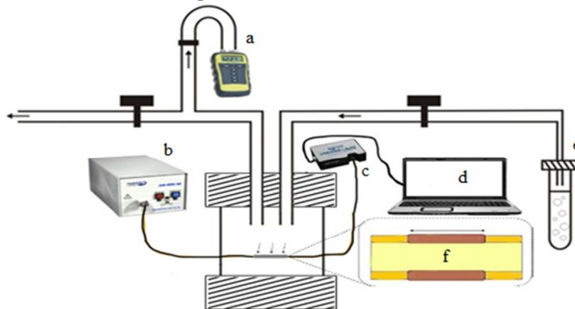
**Figure 3.** Experimental set up of absorbance measurement of methanol
