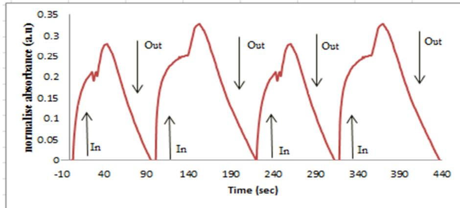
**Figure 8.** Response of the intrinsic sensor of POF to methanol vapour inside the testing chamber.
