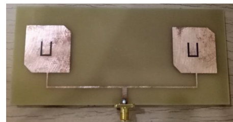
Fig. 9. Truncated corner array microstrip antenna with U Slot
