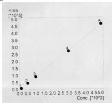
Fig. 2 Cyclamate calibration curve
