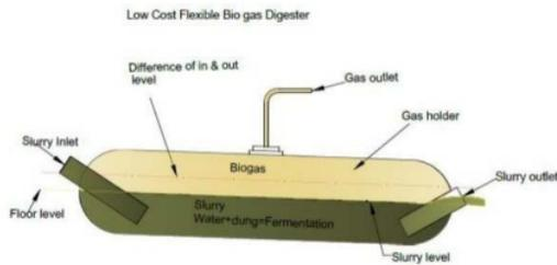
Gambar 6. Digester tipe balon
