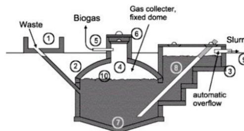
Gambar 4. Digester Fixed Dome (Sumber TBW)
