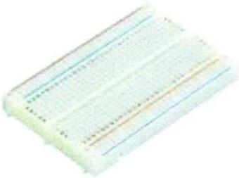
A standard white breadboard used for prototyping electronic circuits, featuring a grid of holes and colored power rails.    |
