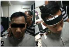
Fig. 2: The sensor placement on the subject's Fp2 location: A. EEG electrode and B. integrated ECVT-EEG sensor
