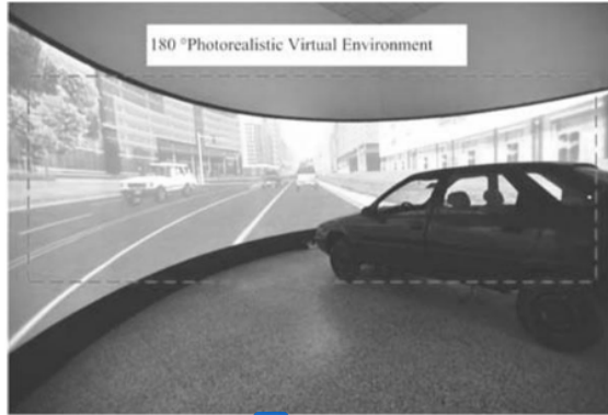
Fig. 1. Driving Simulator of Intelligent Transportation Systems Research Center at Wuhan University of Technology, China
