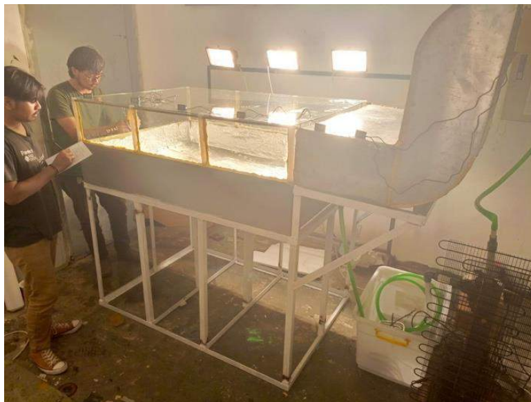
Fig. 1. Forced-flow desalination experimental rig
