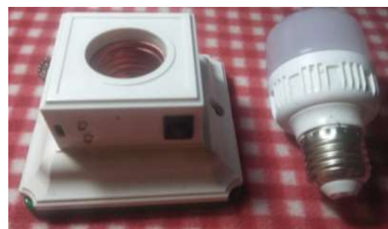
Gambar 2 : contoh lampu emergency
