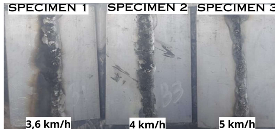
Figure 2 . TIG welding results on aluminum 6061
