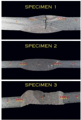
Figure 4. Vickers hardness testing results
