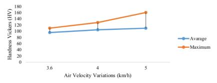
Figure 5. Graph of relation between hardness value and air velocity variation
