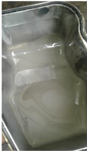
Figure 1. Engine oil contaminated with water
