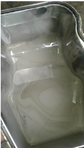
Figure 1. Engine oil contaminated with water
