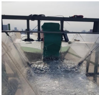
Fig. 1. Dethridge wheel experimental rig installation
