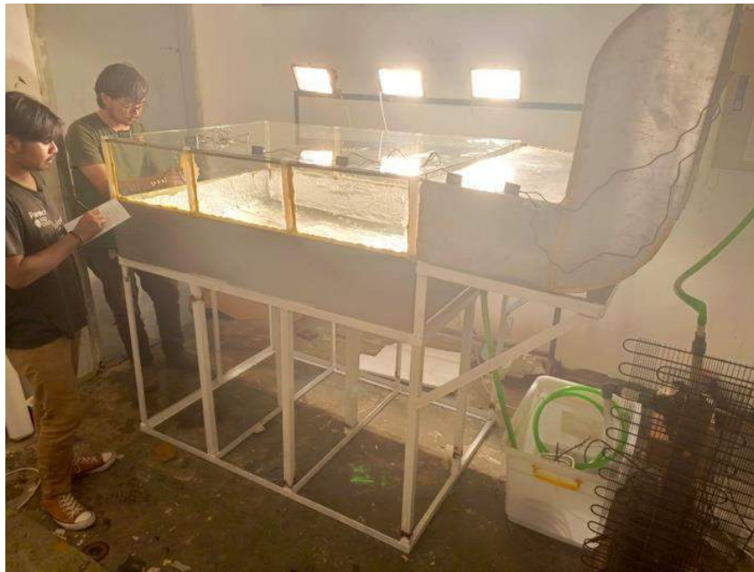
Fig. 1. Forced-flow desalination experimental rig
