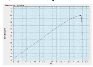
Figure 12. Tensile strength graph of sample KS100
