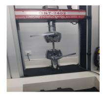
Figure 1. The HT-2402 tensile testing machine
