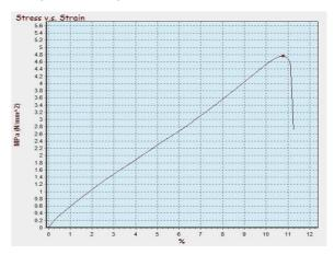
Figure 13. Tensile strength graph of sample KR60KS40
