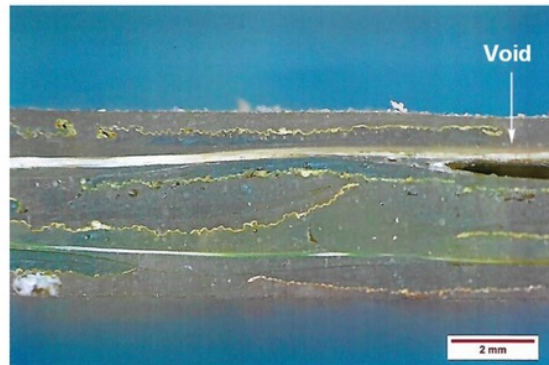
Fig. 3 Cross-sectioned microscopic structure of the RSF-reinforced polymer composite at 30% fibre loading (RSF NaOH ).
