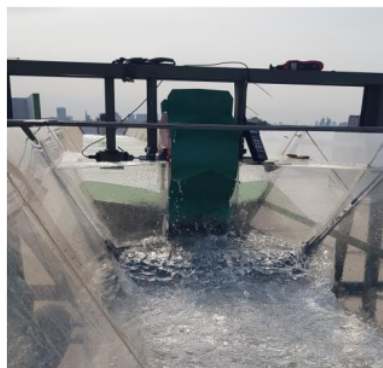
Fig. 1. Dethridge wheel experimental rig installation
