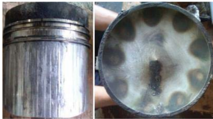
FIGURE 5. Spray injector on piston-cylinder #5
