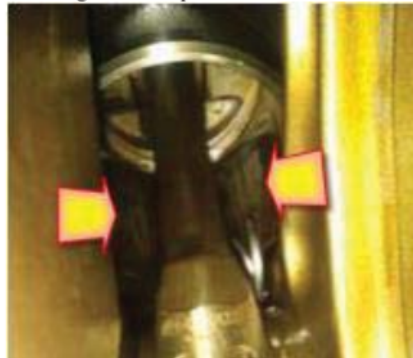
FIGURE 1. Fuel leakage from the liner and piston.
