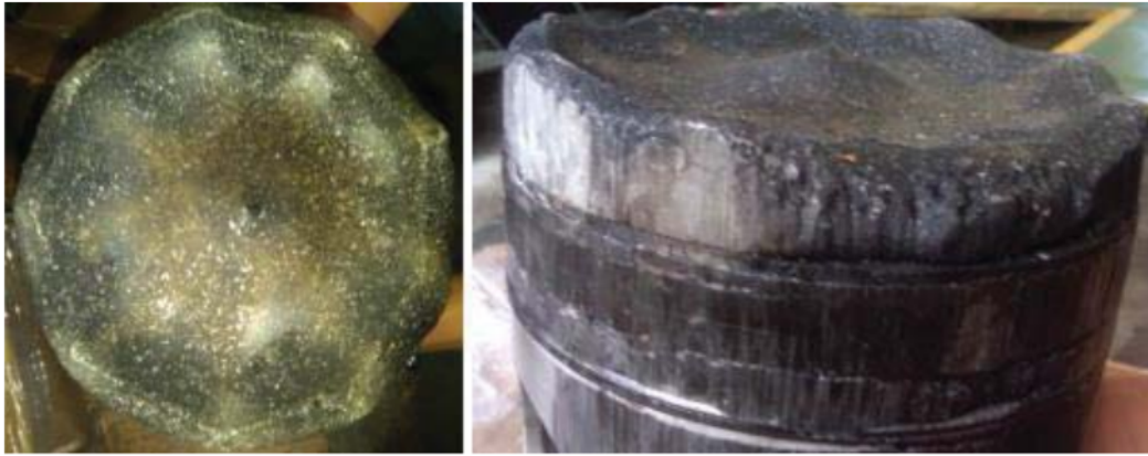
FIGURE 4. Top melting piston crown on cylinder # 12.
