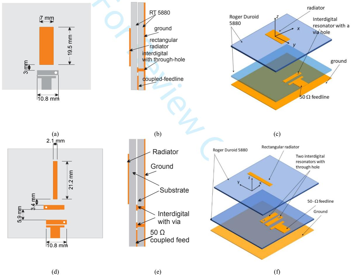
In the co-design of a filtering antenna, radiator extraction is essential because, with various radiator sizes, we can generate the same frequency operation but with different radiation values. Furthermore, the radiation quality significantly affects the operating bandwidth produced by the filtering antenna, which must have the same value as the external quality of a filter in the co-design.
