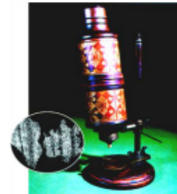
Gambar 1-1. Peralatan Robert Hooke dalam Mengamati Sayatan Tanaman Gabus (Karp, 2013. Cell and Molecular Biology 7 th Edition )
